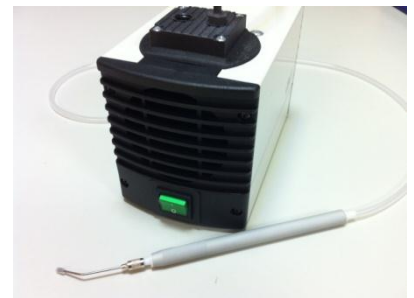
Vacuum Tweezers incl. Vacuum Pump (115-230V, 50-60Hz)
