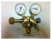
N<sub>2</sub> gas pressure reducer, metric
